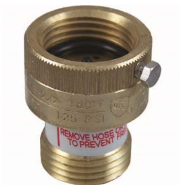
Vacuum breaker, installed on ALL outdoor faucets at Wills Creek – must be kept in place at all times BC Plumbing code requirement for all exterior water connections
