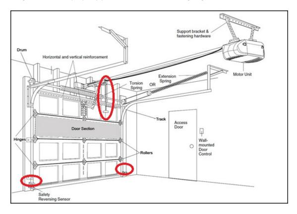
If you have an emergency release cord that hangs down near the door in the closed position, remove the red plastic piece (leaving just the dangling red rope) to prevent criminals from using a coat hanger to release the emergency switch and silently open the door.
